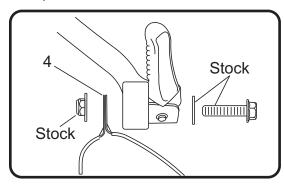
7. Standing behind the motorcycle, check for proper alignment of the muffler.
