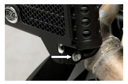
• Fit a cable tie through the bottom left hand location on the guard and secure into place
