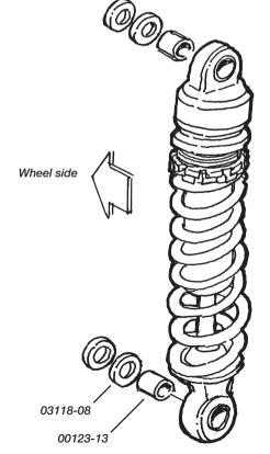
Normaly the shock absorber is mounted with the cylinder head upwards. Check that there is enough clearence to other details both in loaded and unloaded position.
