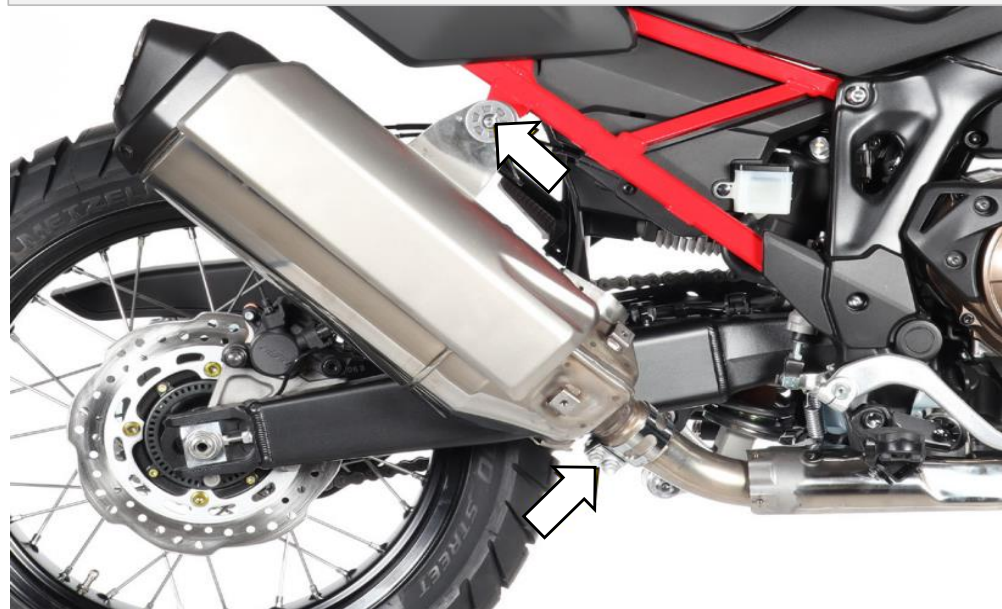
6. Disassemble silencer by loosen marked screw and clamp.
