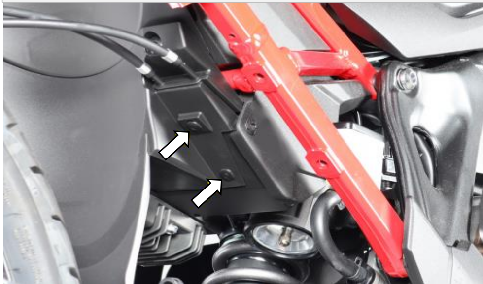
4. Unscrew 4 x marked screws and remove mudguard and servo motor.
