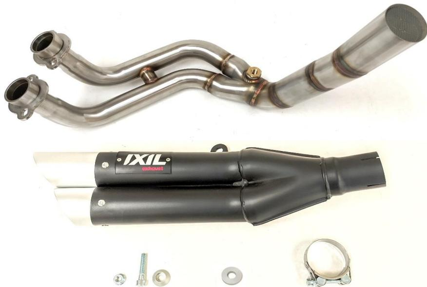
1. Assemble main manifold and just hand tighten 4 x stock cylinder nuts.
