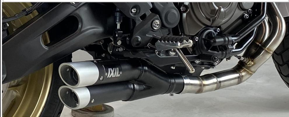
4. Assemble muffler and hand tighten M8x50 screw, screw cover, C5 spacer and M8 nut as shown in the picture. (C5 spacer between frame's bracket and muffler's bracket)
