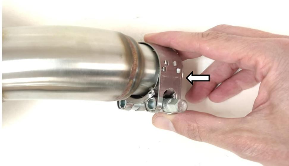
Slip the silencer and link pipe onto stock collector and fasten them to the footrest bracket using 1 x M8x50 screw, 1 x EMBM8 cover screw & 1 x M8 nut.
