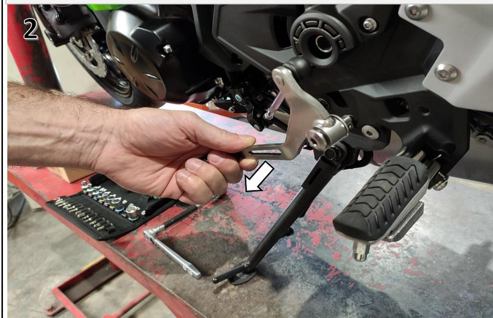
Locate and unscrew pre silencer clamping screw.
