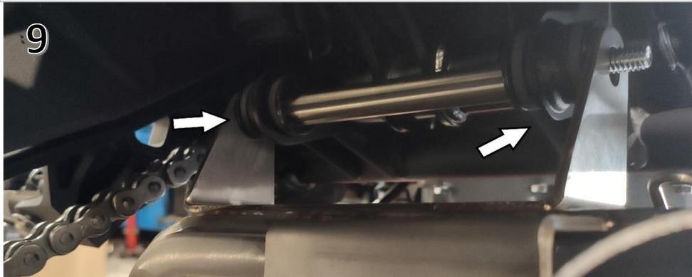
Place both springs using tool from our fitting kit.
