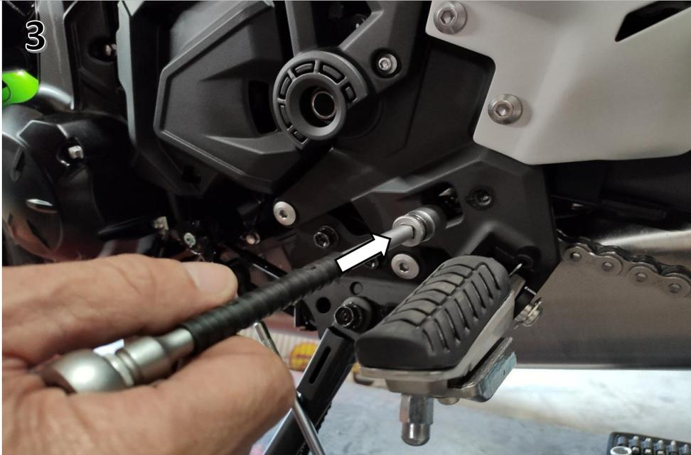
Once the screw is removed all the stock exhaust system may fall and cause injuries. Please hold it carefully.
