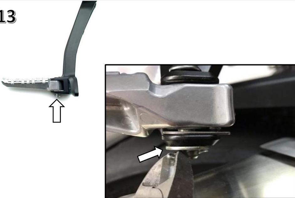
Replace stock pin with 1 x M6x45 screw, 1 x ARAN M6A & M6 nut to hold silencer.
