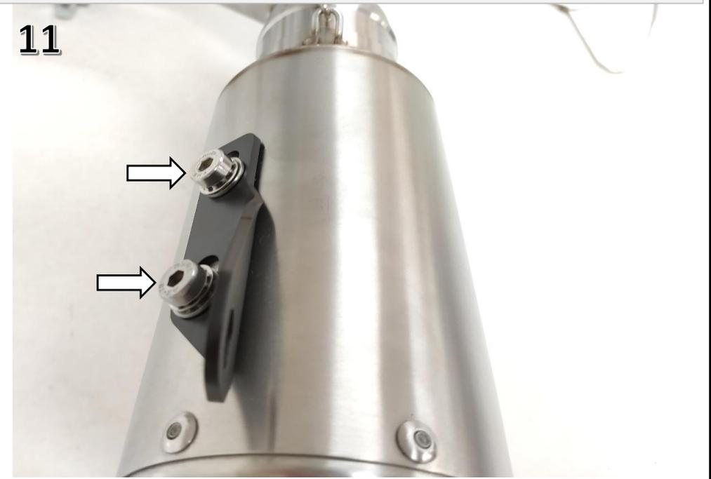
Place SOP9680 BRACKET using 1 x M8x16 SCREW, 1 x ARAN M8 WASHER & 1 x M8 NUT.
