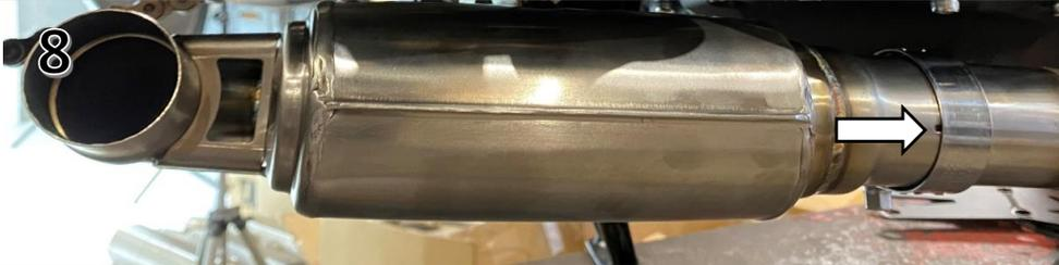
Use 1 x M8x150 SCREW & 1 x M8 NUT to hold and tighten the cat box to the main frame bracket.
