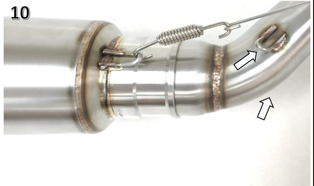
Correctly position SOP9262 BRACKET using 2 x M8x16 SCREW, 2 x ARANM8 WASHER & 2 x GLOW M8 WASHER.
