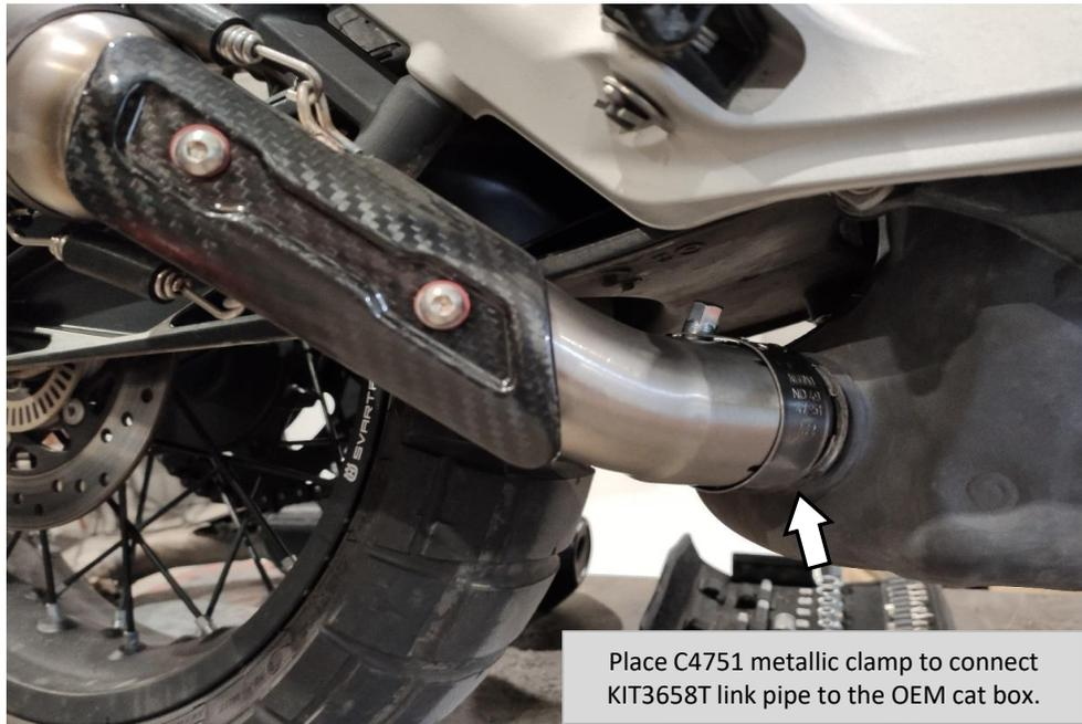
Place C4751 metallic clamp to connect KIT3658T link pipe to the OEM cat box.
