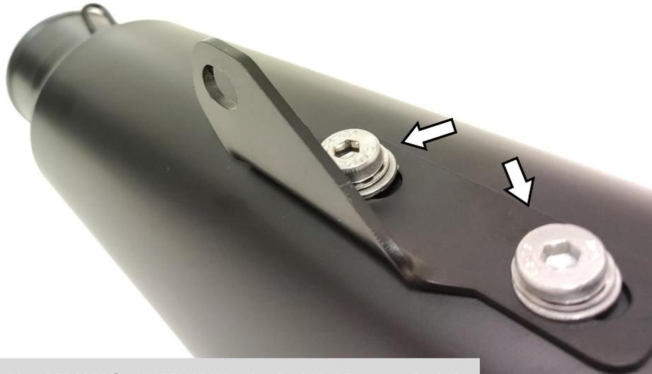
Position SOP6278 for HUSQVARNA using 2 x M8x16 screws, 2 x M8 washer & 2 x M8 GLOW washers as shown.
