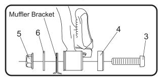
4. Torque (No. 3) *M8X45*, 8mm bolt to 23 Nm (2.3 kg-m, 17 ft-lbs).
