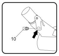
2. Install (No. 4) *HT SHLDR77*, muffler clamp heat insulator onto (No. 3) *MCYM5-CCBX(-X)*, muffler clamp.
