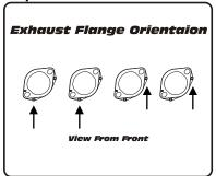
2. Install springs onto flanges, noting spring hook locations of header.
