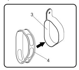
2. Slide (No. 5) 27-59M, exhaust clamp over (No. 1) 12551-435, tailpipe inlet. Install (No. 1) 12551-435, tailpipe inlet over the stock header outlet.
