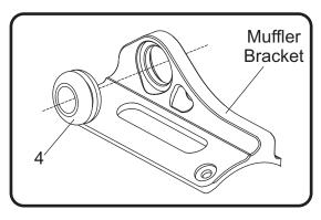
4. Carefully slide Yoshimura muffler assembly over the stock header outlet. Secure muffler to (No. 1) 13120-BRKT, muffler hanger bracket using the hardware provided in the kit. Orientation is as follows: (No. 6) M8X30H, 8mm bolt, (No. 5) ALS-003, aluminum spacer, (No. 9) muffler, (No. 1) 13120-BRKT, muffler hanger bracket, and (No. 7) 8MMNUT, flange nut. See diagram below.
