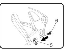
2. Align (No. 5) *13141-RMBKT*, muffler bracket adapter to the backside of the right footpeg bracket. Secure using the stock bolt.
