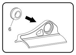
5. Install (No. 7) *ALS-003*, aluminum spacer into (No. 6) *Z1022*, rubber grommet.
