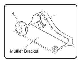
2. Install (No. 5) *ALS-003*, aluminum spacer into (No. 4) *Z1022*, rubber grommet as shown.
