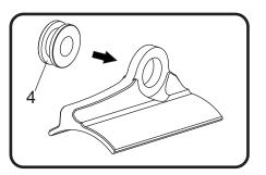
7. Install (No. 7) ALS-047 for Husqvarna OR ALS-056 for KTM, aluminum spacer in the backside of (No. 4) Z1023, rubber grommet and install (No. 5) ALS-046, aluminum spacer in the frontside as shown below.
