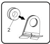
Install (No. 3) ALS-046, aluminum spacer in the front side of (No. 2) Z1023, rubber grommet and install (No. 4) ALS-054, for Husqvarna OR ALS-057 for KTM aluminum spacer in the back side of (No. 2) Z1023, rubber grommet as shown below.
