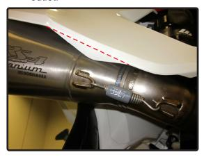
6. Torque muffler mount bolts to factory specification.
