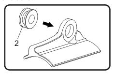
4. Install (No. 5) ALS-047 for Husqvarna OR ALS-056 for KTM, aluminum spacer in the backside of (No. 2) Z1023, rubber grommet and install (No. 3) ALS-046, aluminum spacer in the frontside as shown below.
