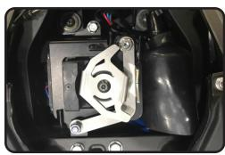
2. Firmly hold servo pulley in place and remove tamper proof torx bolt using the proper torx bit. Install (No. 6) 1464-CKRPLT, servo motor stopper plate on top of the stock pulley as shown above and secure using the stock torx bolt.
