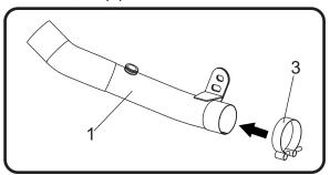
Install (No. 1) 14182-714, tailpipe over the stock header outlet and align tailpipe chassis mount bracket to chassis mount. Secure using the stock chassis mount bolt and (No. 5) 10MMFNUT, flange nut. Do not torque at this time.
